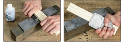
On the lapping plate the blade is worked with silicon carbide powder and water under high pressure. For easy pressure distribution a piece of wood will serve best. The powder grinds into a fine paste that has an additional polishing effect. The back is normally only trued once on brand-new tools using flat, trued hones. After that, the back is only honed on a fine sharpening stone.
