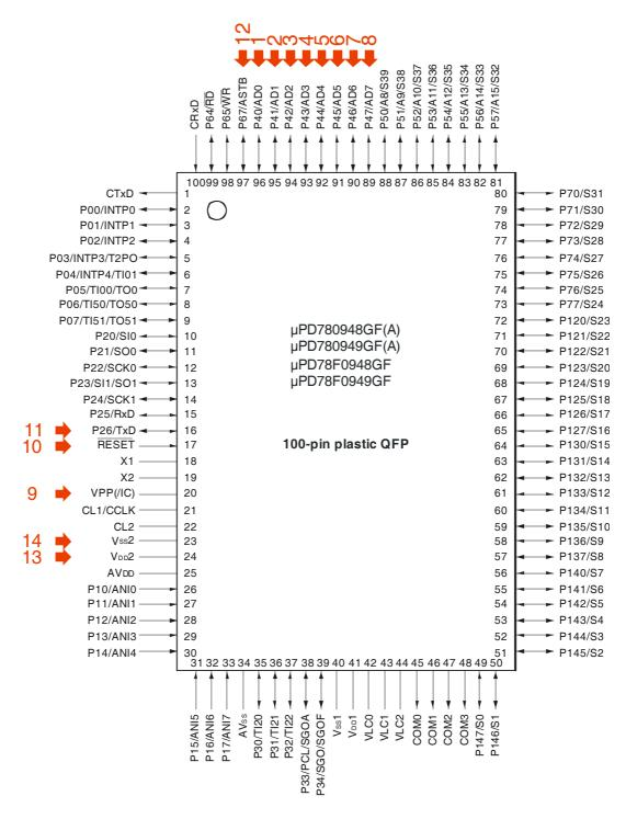
Figure 3. In-Circuit wiring diagram for uPD78(F)0948/49 MCU
