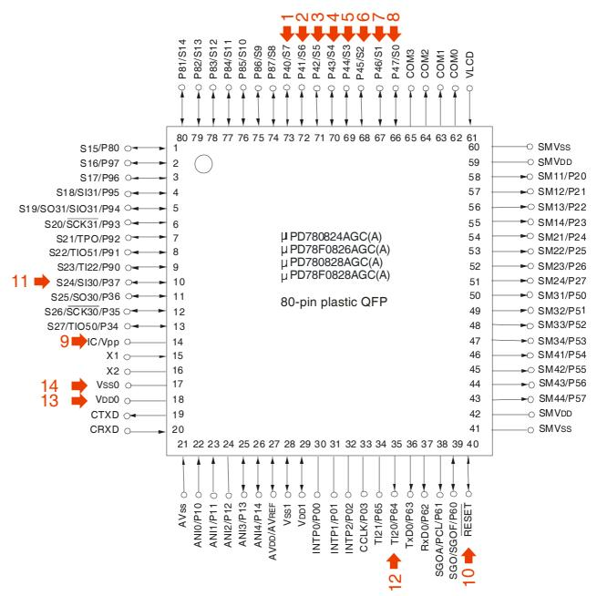
Figure 4. In-Circuit wiring diagram for uPD78(F)0828A MCU
