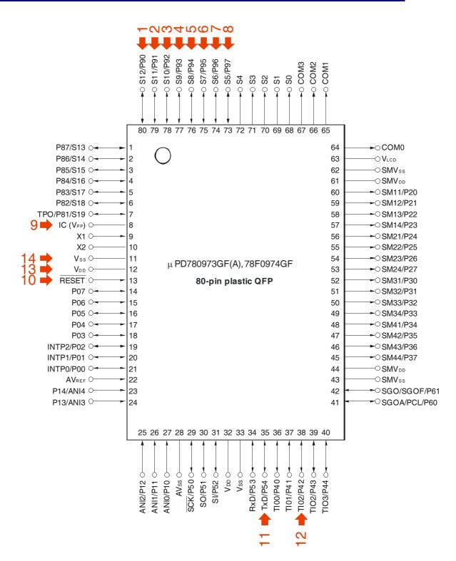
Figure 2. In-Circuit wiring diagram for uPD780973 MCU
